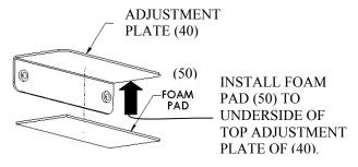
Figure 4. Install Pads on Adjustment Plates
